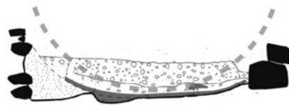
Suggested Cross-section of Boat Length 5.5 - 6 m, Max. Width 90 cm from Van de Moortel 2012, 18 Fig 3.4
